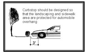
required for all head-in parking spaces adjacent to landscaped areas. Wheel stops shall be designed so that the overhang of vehicles is contained totally within the parking space. When wheel guards are used, they shall be centered 3 feet from the property line for 90 degree parking, 2.3 feet for 60 degree parking, and 2.0 feet for 45 degree and 30 degree parking.
